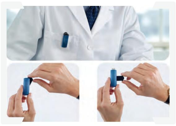
To open your device, hold the clip and turn 180 degrees to either side to extend the USB connector.
