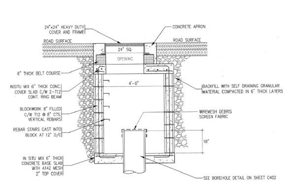
3 TYPICAL BOREHOLE CROSS-SECTION M2 N.T.S.
