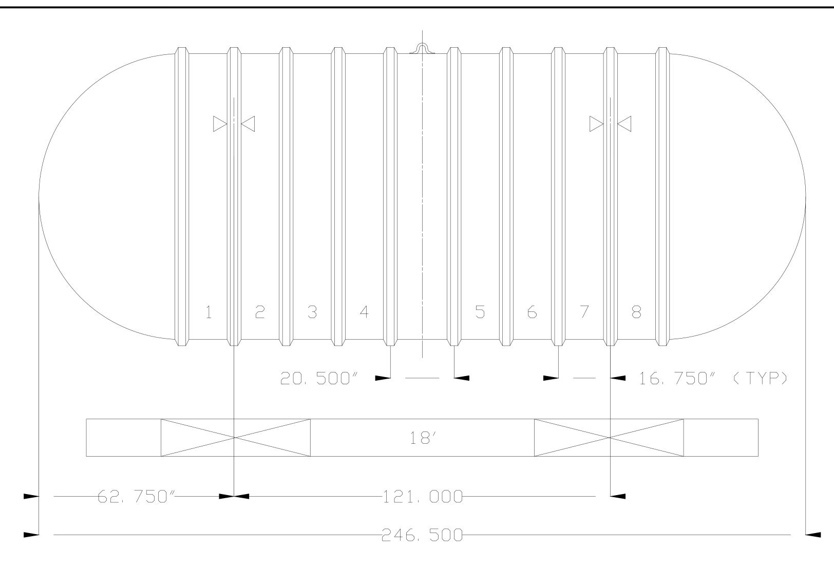
1 SINGLE-WALL 5000 GALLON SEPTIC TANK, 8' DIA. M2 N.T.S.
