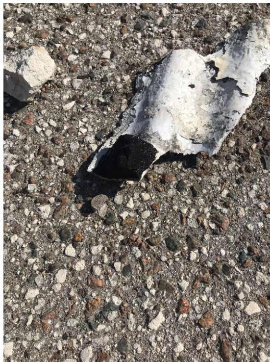
Sample KOBE 1B – Building A Roofing West – 20% Chrsotile
