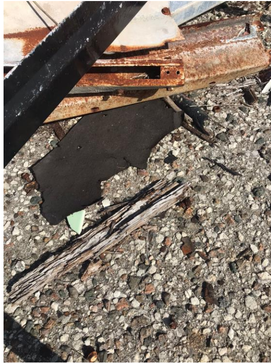
Sample KOBE 4B - Building A Tar Paper – No asbestos
