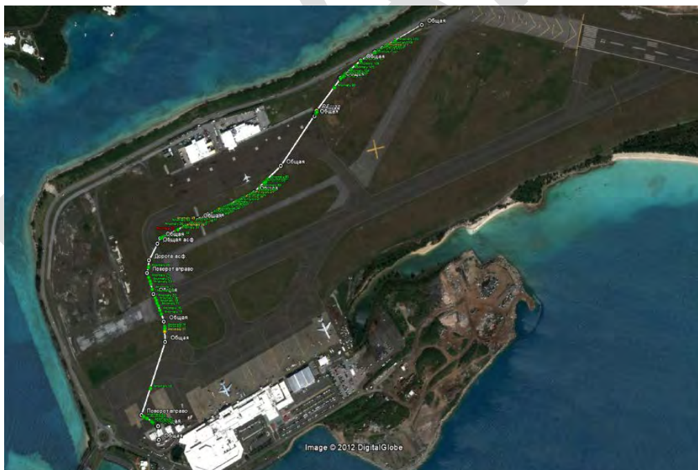
Figure 3 – Map of the Bermuda Airport Supply Jet Fuel Pipeline
