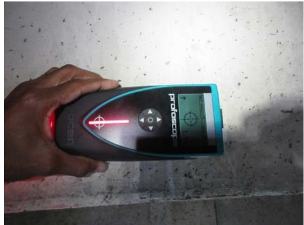
Photo 5.1.10. Rebar scan of B1.
