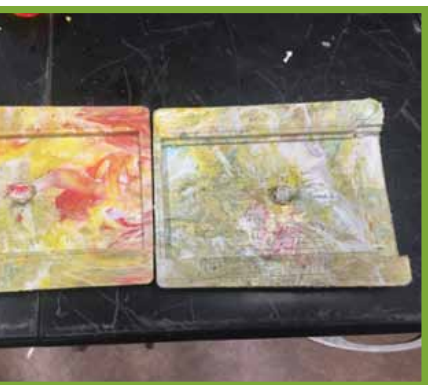
Marbleized plastic cell phone charger cover produced from CNC mold
