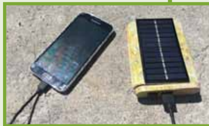
Fully assembled prototype of solar powered cellphone charging case from recycled plastics.
